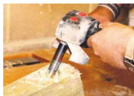
▲ On softer, wet timber the TurboShaft struggled to cut
